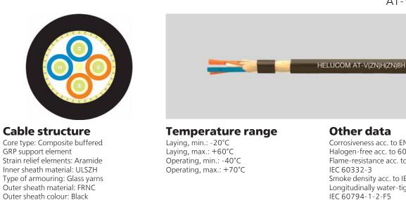
Other data Corrosiveness acc. to EN50267-2-3 Halogen-free acc. to 60754-2 Flame-resistance acc. to IEC 60332-1 and IEC 60332-3 Smoke density acc. to IEC 61034 Longitudinally water-tight acc. to IEC 60794-1-2-F5 UV-resistant Resistant to hammer impact acc. to IEC 60794-1-2-E4 Oil-resistant
