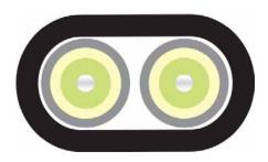
**Cable structure** Core type: Tight buffer Strain relief elements: Aramide Outer sheath material: PVC Outer sheath colour: Black
